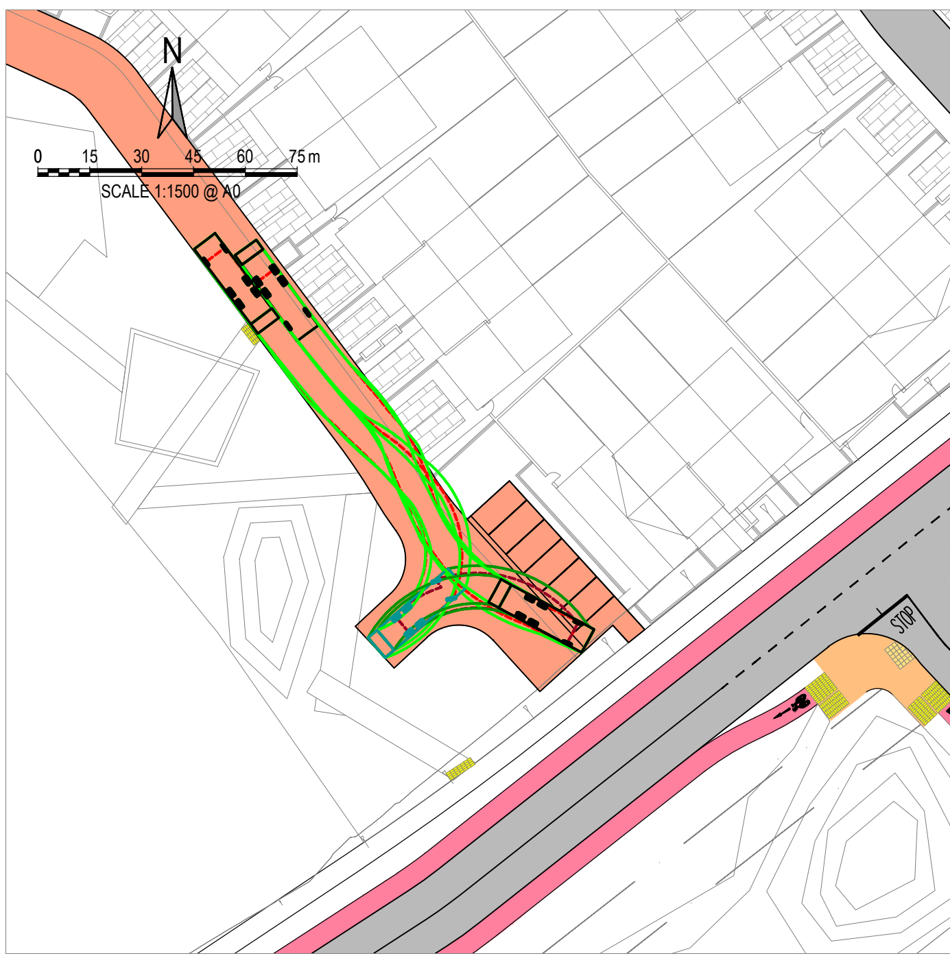
3 REFUSE VEHICLE AT HAMMERHEAD Scale 1:500
