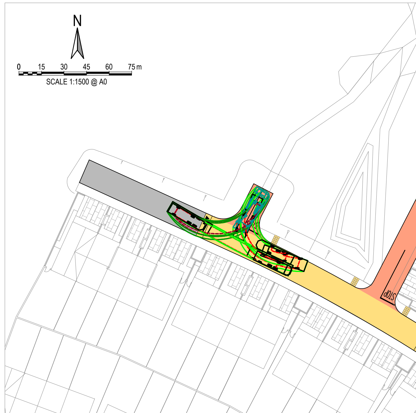
4 REFUSE VEHICLE AT HAMMERHEAD Scale 1:500
