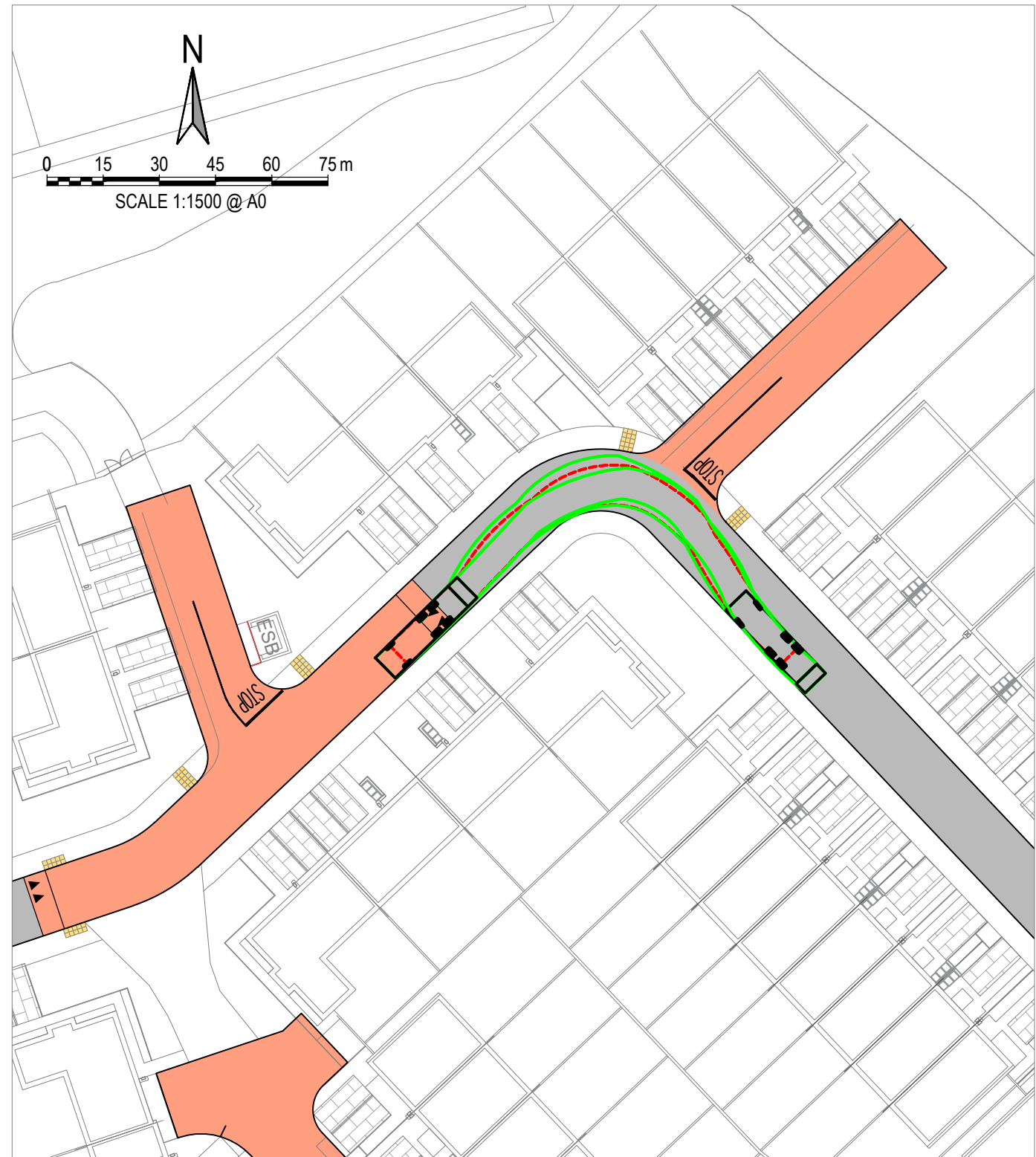
8 REFUSE VEHICLE AT BEND Scale 1:500
