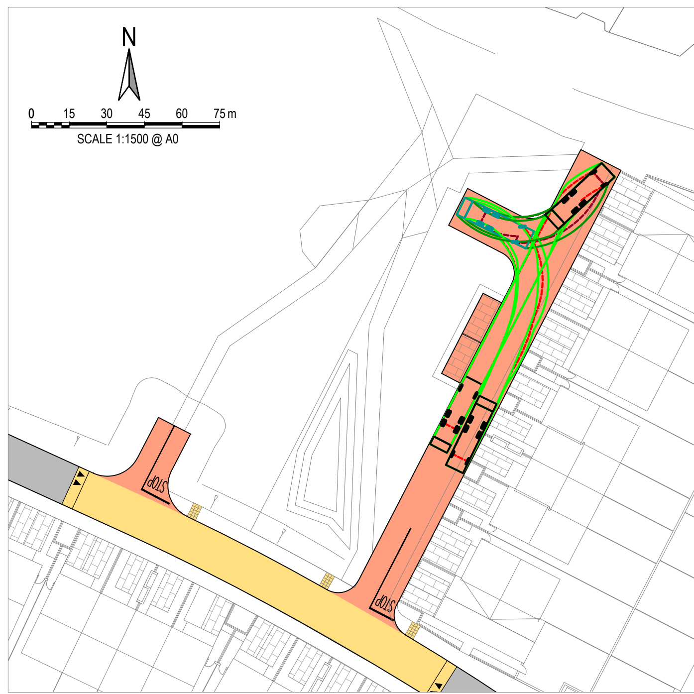
1 REFUSE VEHICLE AT HAMMERHEAD Scale 1:500
