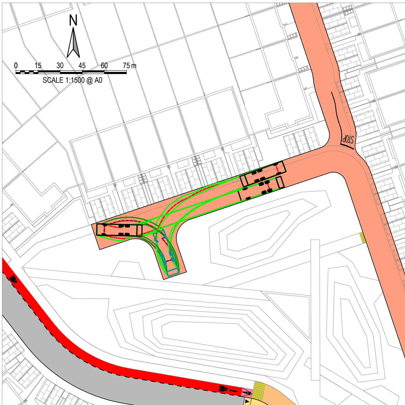
5 REFUSE VEHICLE AT HAMMERHEAD Scale 1:500
