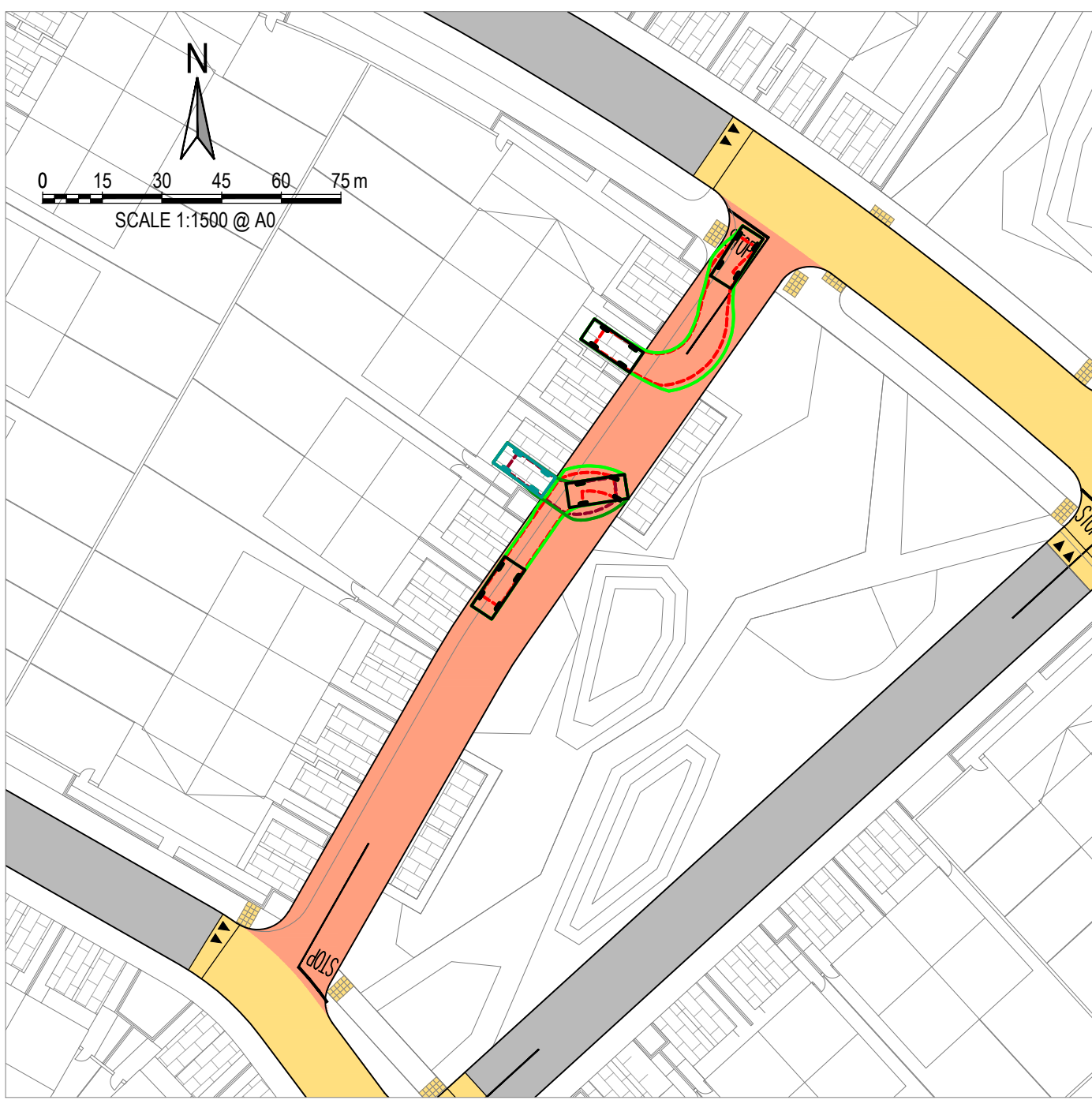
2 4x4 VEHICLE ENTERING AND EXITING DRIVEWAY Scale 1:500
