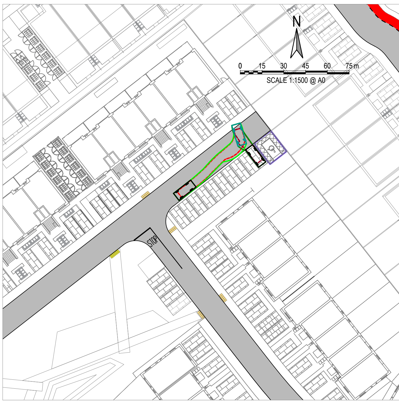
4 4x4 VEHICLE AT HAMMERHEAD Scale 1:500
