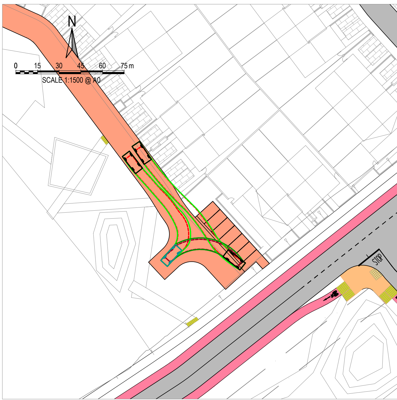
3 4x4 VEHICLE AT HAMMERHEAD Scale 1:500
