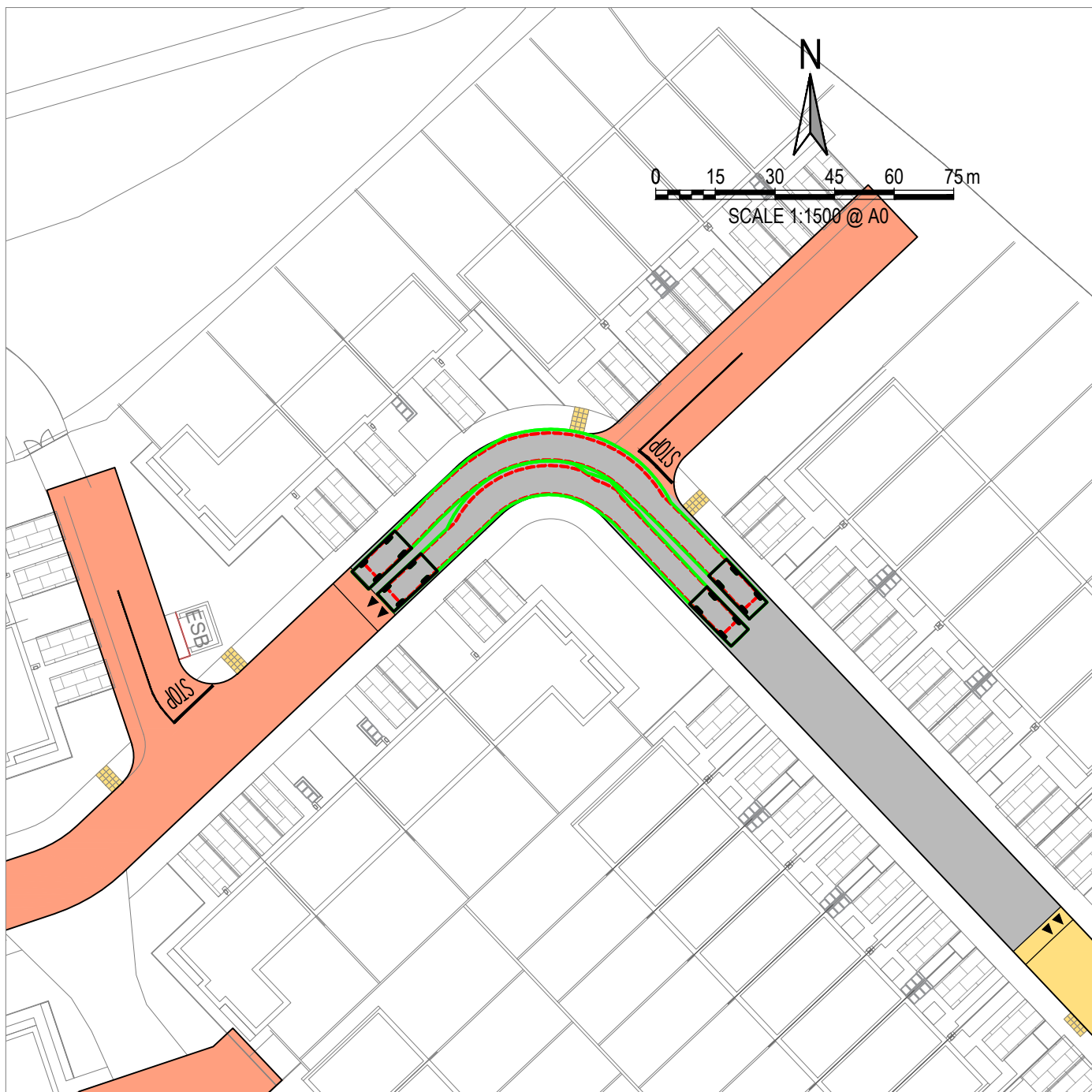
5 4x4 VEHICLE AT BEND Scale 1:500
