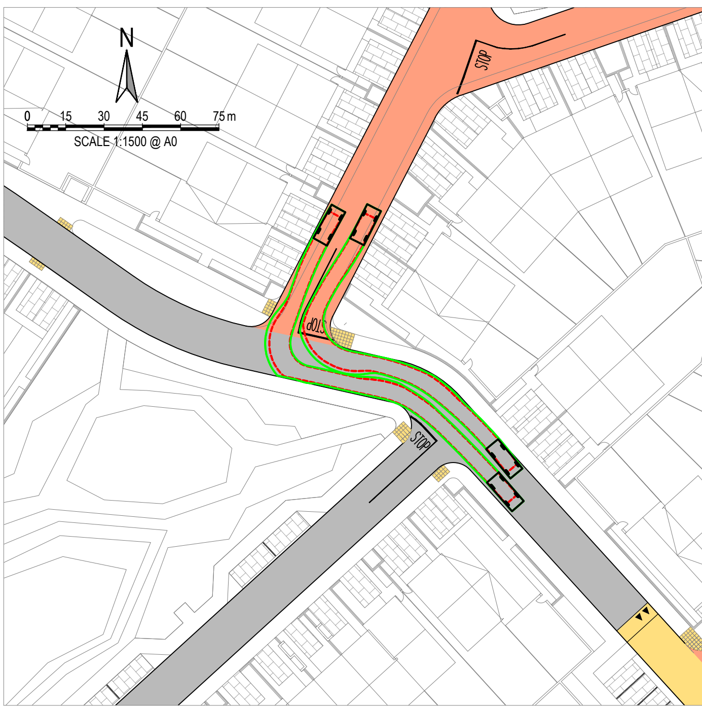
1 4x4 VEHICLE AT BEND Scale 1:500
