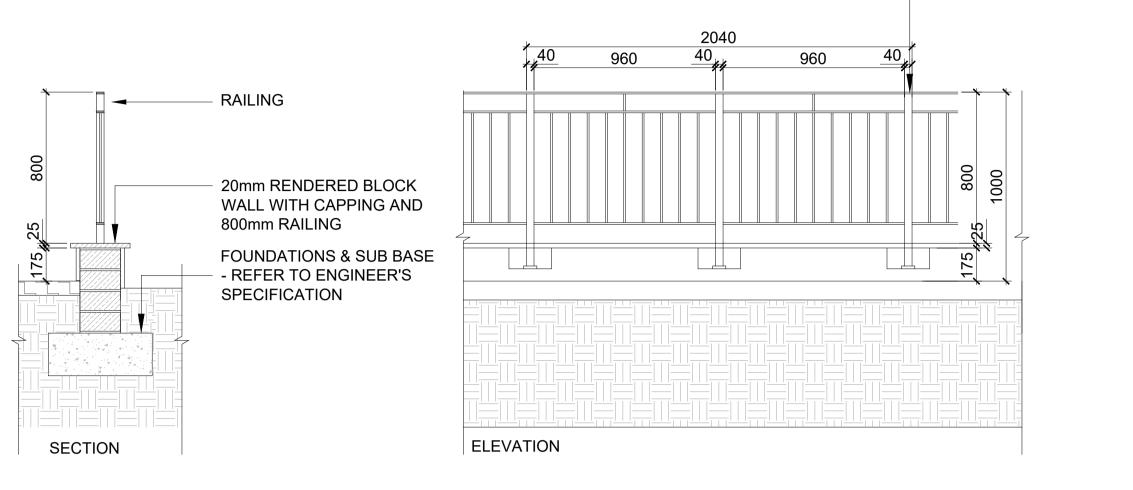
O1 TYPICAL DETAIL : 2.0M HIGH RENDERED CONCRETE BLOCK PIER TO PUBLIC OPEN SPACE SCALE: 1:20 @A1
