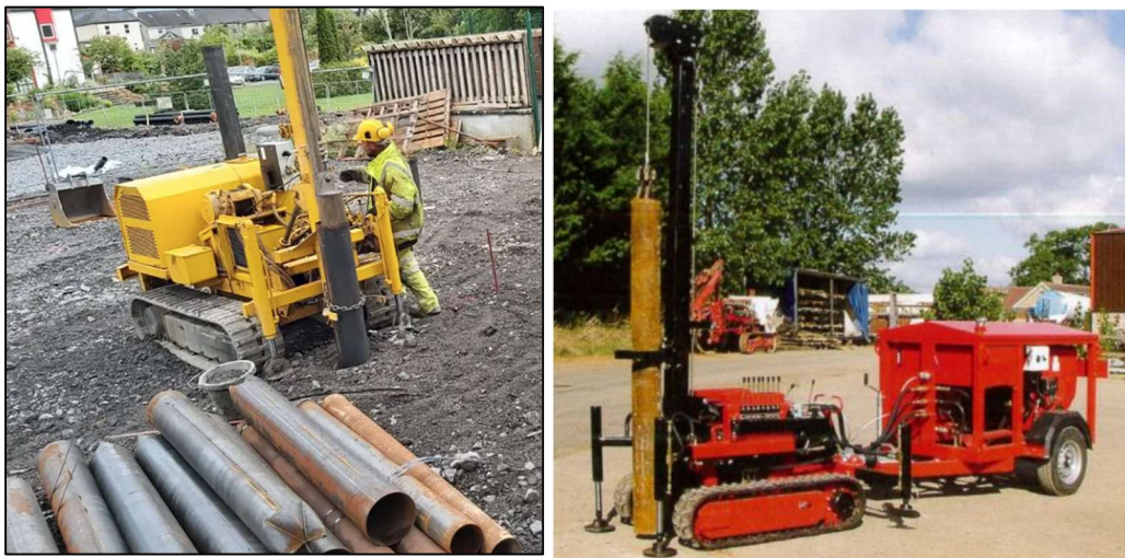
Figure 10: Typical Mini-Piling Rigs for bottom end driven steel piles
