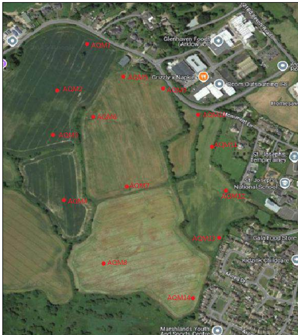
Figure 9.2: Baseline Air Quality Monitoring Locations AQM1 TO AQM15 Dust Levels Tested with DustTrak II Aerosol Monitor 8530.
