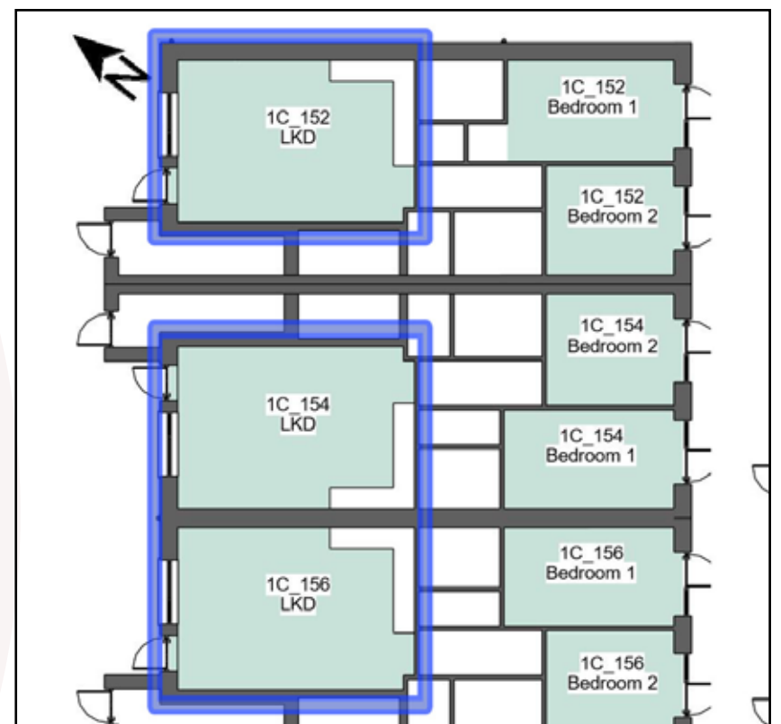
Figure 5.2: Example of non compliant LKD of duplexes.
