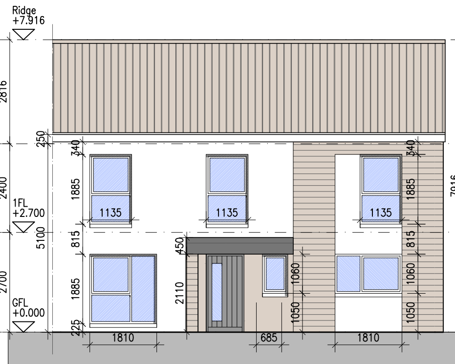
12 Type F2 - Front Elevation [Character Area 1C] 207 1:100@A1 3 BED HOUSE
