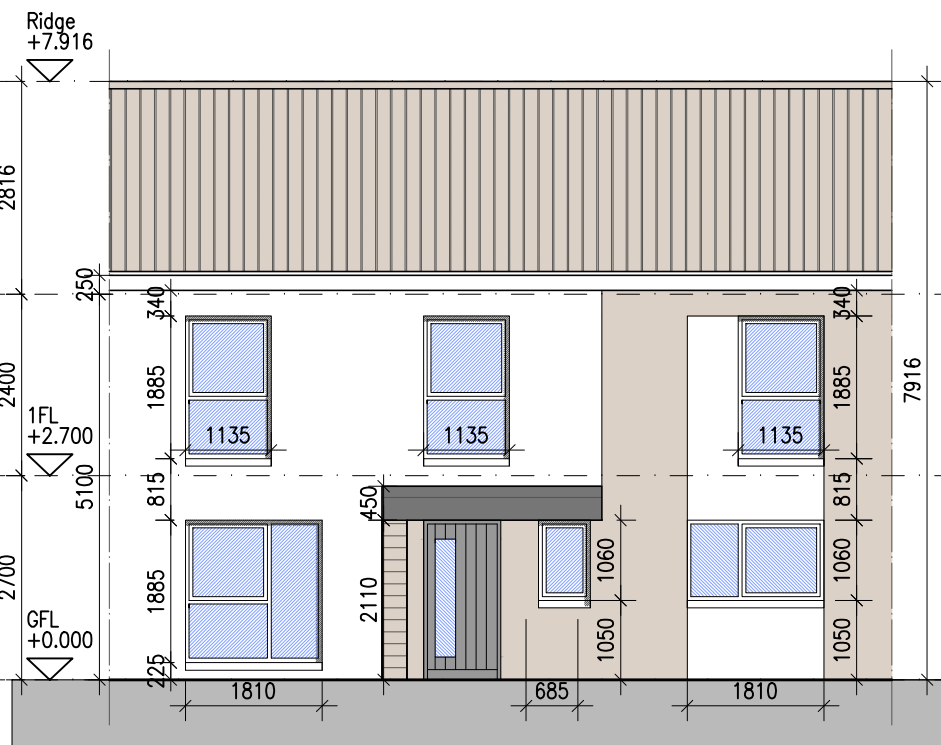
05 Type F1 - Front Elevation [Character Area 1C] 207 1:100@A1 3 BED HOUSE
