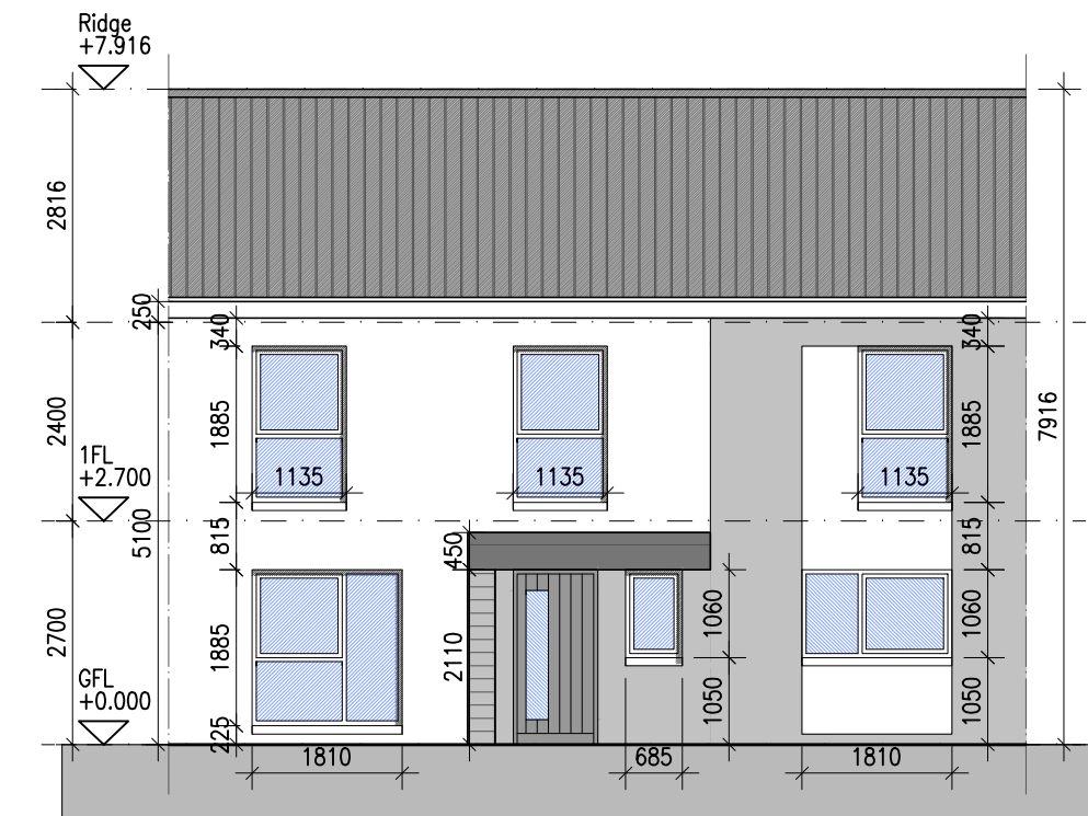
04 Type F1 - Front Elevation [Character Area 1B] 207 1:100@A1 3 BED HOUSE
